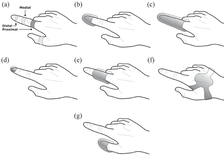
Fig. 4. FAD form factors: (a) rings, (b) distal addendum, (c) whole finger addendum, (d) fingernail addendum, (e) sleeve, (f) palm component that accompanies an FAD, and (g) thumb addendum.
