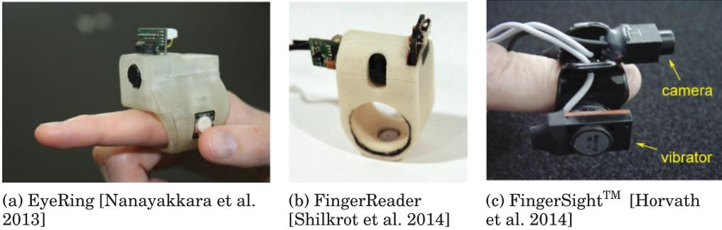
Fig. 7. Finger-worn cameras. Images courtesy of authors.
