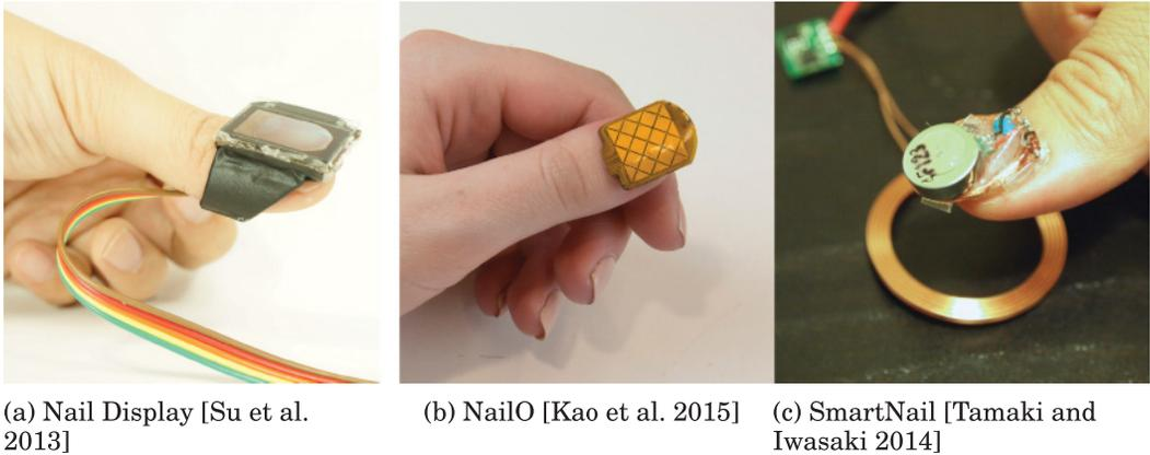
Fig. 5. Fingernail-augmenting devices: (a) a miniature display added to the thumb, (b) a touch-sensitive pad for 2D cursor control, and (c) a radio-controlled vibration motor.
