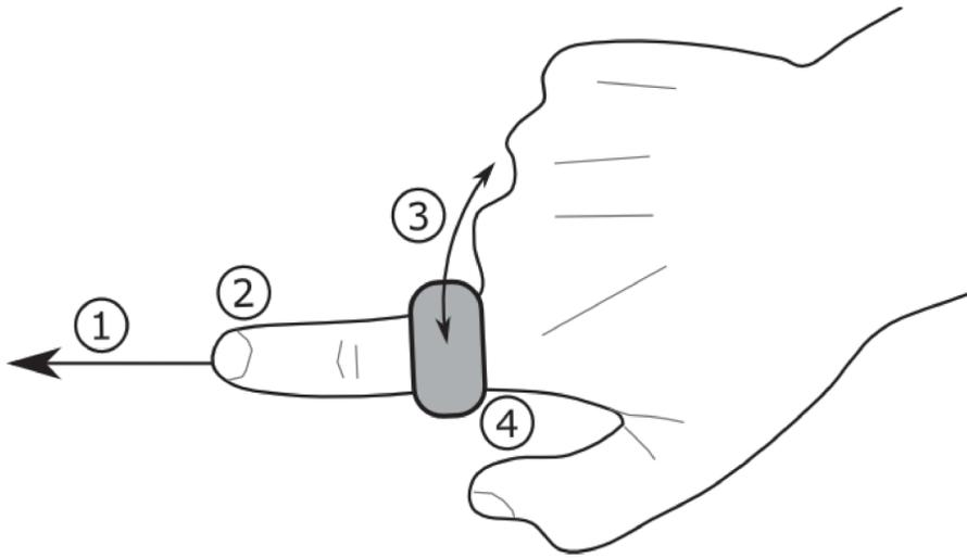
Fig. 8. Types of FAD actions: (1) pointing/external, (2) touching/on surface, (3) gesturing, and (4) clicking/touching on device.
