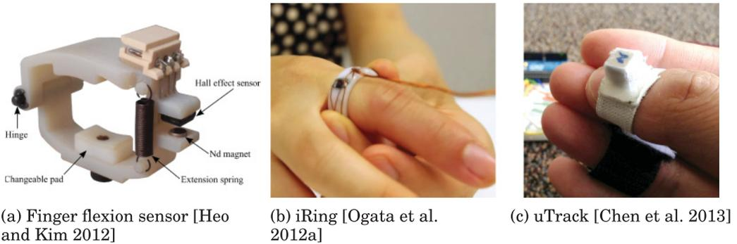
Fig. 6. Input modalities in finger-worn devices: (a) a sensor for the flexion of finger tendons, (b) an IR reflectance sensor for different parts of the finger's skin, and (c) a magnetic sensor. Images courtesy of authors.
