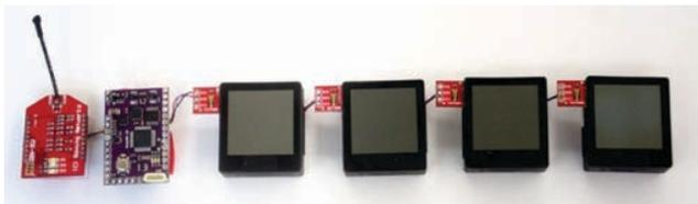
Figure 2. The hardware setup consists of four interconnect displays, each equipped with a light sensor to detect movements of the sleeve. An IMU measures the arm's orientation.
