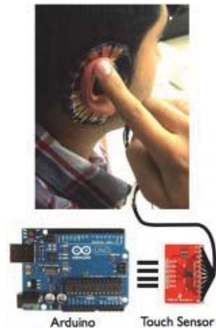
Figure 2: Hardware apparatus used in the controlled experiment.
