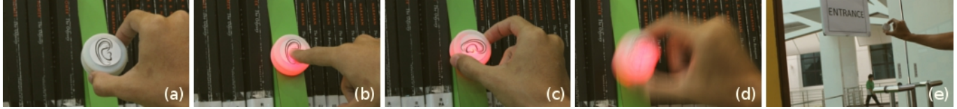
Figure 1. StickEar prototype: (a) Deploy on an object. (b) Press to activate. (c) Rotate to tune. (d) Shake to reset (e) Redeploy on another object.
