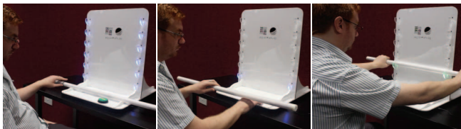
Figure 3. Typical usage of SHRUG (a) Place the pole on the platform for identification (b) Select the game using the selection button on the platform (c) Place the pole on the platform hooks as required by the game
