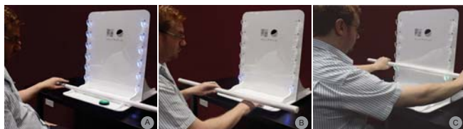
Figure 5. Typical usage of SHRUG (a) Place the pole on the platform for identification (b) Select the game using the selection button on the platform (c) Place the pole on the platform hooks as required by the game
